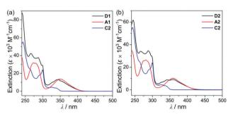
Fig. 2 (a) UV-vis absorption spectra in THF (5.0  $\times$  10<sup>-5</sup> M) for (a) **D1**, **A1**, and **C2** and (b) **D2**, **A2**, and **C2**.
