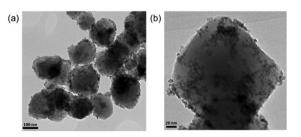
Fig. 1 (a) and (b) HR-TEM images of fresh Pd-Pt-Fe<sub>3</sub>O<sub>4</sub> NPs.
