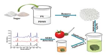
**Scheme 1** Schematic synthesis and applications of PDMS sponge-SERS substrate.
