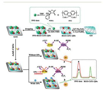
Fig. 24 Double-potential ratiometric ECL for organophosphorus pesticides (OPs) analysis. (Reprinted with permission from ref. 117. Copyright 2017, American Chemical Society.)
