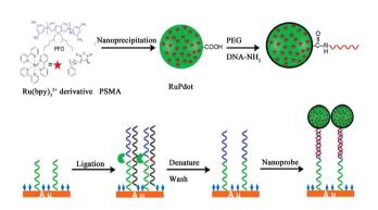
Fig. 16 Schematic diagrams of (A) Preparation of RuPdots nanoprobe using PFO, hydrophobic  $\mathrm{Ru}(\mathrm{bpy})_3^{2+}$  derivative, and PSMA; (B) SNP detection with ligase detection reaction and nanoprobe. (Reprinted with permission from ref. 78. Copyright 2017 American Chemical Society.)
