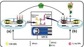
Fig. 26 Schematic illustration of the ratiometric ECL array for CAP quantification. (Reprinted with permission from ref. 89. Copyright 2015,
