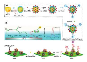
Fig. 15 Schematic illustration of ECL aptasensor preparation process and possible luminescence mechanism: (A) fabrication of  $TBA_2$ -(AuNPs-Sem)<sub>n</sub>-AuNCs signal probe; (B) fabrication of CdTe QDs@C60 NPs, and (C) possible ECL mechanism of the QD-based ECL system. (Reprinted with permission from ref. 77. Copyright 2015 American Chemical Society.)
