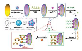
Fig. 21 Schematic diagram of the preparation of the ECL aptasensor. (Reprinted with permission from ref. 92. Copyright 2015, Elsevier.)
