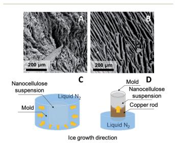
Fig. 6 SEM images of horizontal cross-section of CNF (A) and CNC (B) foams obtained by homogeneous freezing (C) and unidirectional ice templating (D), respectively (adapted from Munier et al.60 Reproduced with the permission of ACS Publications).
