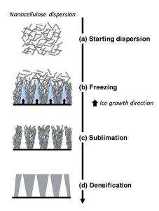
Fig. 5 Schematic diagram of directional ice-templating of nanocellulose dispersion (adapted from Deville<sup>56</sup>).
