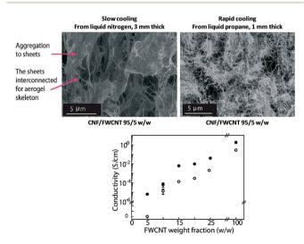
Fig. 11 Influence of cooling temperature on the electrical conductivity of CNF/FWCNT (few walled carbon nanotubes) foams produced by homogeneous freezing. The conductivity of foams frozen either in liquid nitrogen or in liquid propane are represented by the full black and hollow dots, respectively (adapted from Wang et al.88 Reproduced with the permission of Wiley Online Library).
