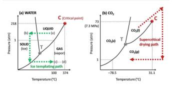
Fig. 4 Phase diagrams of (a) water and (b) carbon dioxide (CO<sub>2</sub>). The critical and triple points are represented on the diagram by the letter C and T, respectively. The phase evolution of water and CO2 during ice sublimation and supercritical drying processes, respectively, are shown by the dashed arrows. The (a) to (d) steps on the water phase diagram corresponds to the ice templating principles detailed in Fig. 5.
