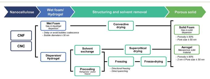
Fig. 1 From nanocellulose to nanocellulose-based foams and aerogels: terminology and processing
