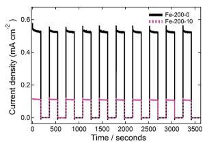
Fig. 8 Stability testing data for the fabricated Fe-200-y photoanodes. The incident simulated-solar radiation was chopped on or off every 3 minutes for a total of one hour, whilst the photoanodes were held at a constant potential of 0.22 V vs. Ag/AgCl (1.25 V vs. RHE).
