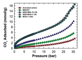
Fig. 7 Comparison of the  ${\rm CO_2}$  adsorption capacity of different materials.
