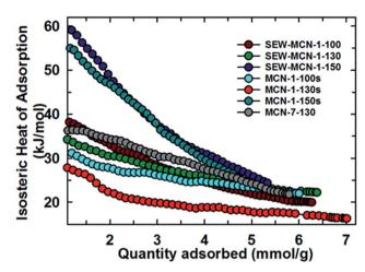
Fig. 8 Variation of isosteric heat of adsorption of SEW-MCN-1-T samples with the quantity of  ${\rm CO_2}$  adsorbed and its comparison with other materials.
