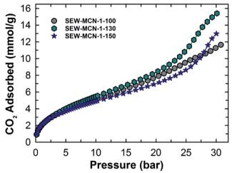
Fig. 6 CO<sub>2</sub> adsorption isotherms of SEW-MCN-1-T samples at 273 K.
