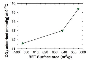
Fig. 9 Relation between the specific surface area and the  ${\rm CO_2}$  adsorption capacity of SEW-MCN-1-T samples.
