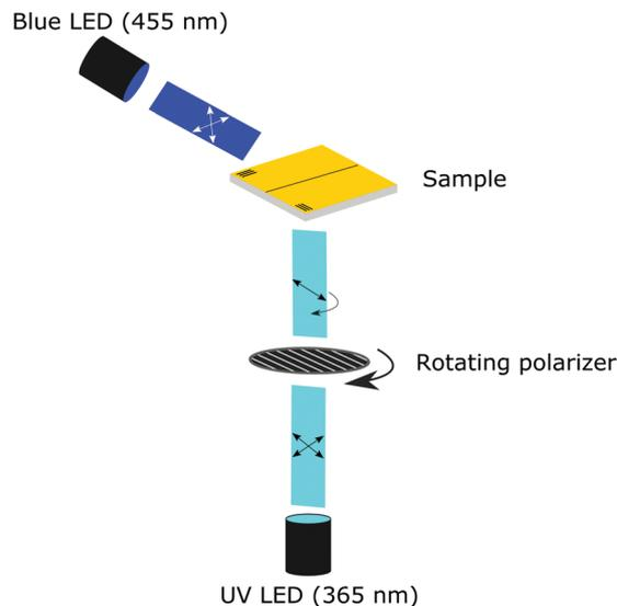
**Fig. 1** Simplified illustration of the illumination setup used for polarized light actuation. Blue light (455 nm) illumination originates from the top and UV light (365 nm) illumination from the bottom while passing through a rotating polarizer. The black lines in the sample indicate the orientation of the director.
