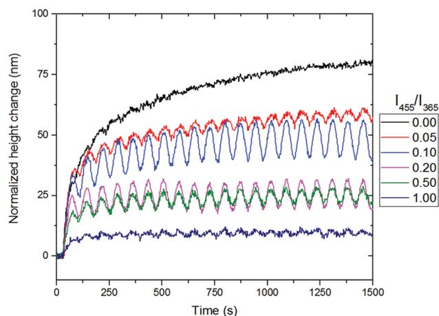
**Fig. 7** The influence of the ratio between the intensity of blue (455 nm) and UV light (365 nm) for the  $0^\circ/90^\circ$  designed coatings with the phase snapshot of the coatings. The comparisons shown in the graph correspond to zone 1 in Fig. 4.
