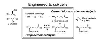
Scheme 1 The current biocatalytic synthesis of adipic acid from glucose requires chemical hydrogenation of unsaturated six-carbon dicarboxylic acids *e.g. cis,cis*-muconic acid or 2-hexenedioic acid.
