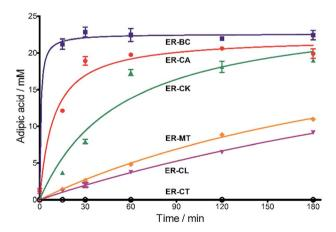
Fig. 1 Time course for the biotransformation of 2-hexenedioic acid into adipic acid by *E. coli* cells expressing ERs. A mixture of *cis-* and *trans-*isomers of 2-hexenedioic acid (20 mM) was used as a substrate. The formation of adipic acid was analyzed using HPLC. ( $\blacksquare$ ) = ER-BC, ( $\bullet$ ) = ER-CA, ( $\blacktriangle$ ) = ER-CK, ( $\bullet$ ) = ER-MT, ( $\blacksquare$ ) = ER-CL, and (O) = ER-CT.
