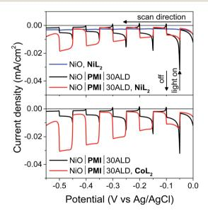
Fig. 4 Linear sweep voltammetry measurements with 10 s light on/off cycles on a NiO working electrode with 0.5 mM NiL<sub>2</sub> (blue) and on a single NiO|PMI|30ALD working electrode without catalyst (black) and with 0.5 mM NiL<sub>2</sub> or 0.5 mM CoL<sub>2</sub> (red) (conditions: 0.1 M H<sub>2</sub>SO<sub>4</sub> and 0.1 M Na<sub>2</sub>SO<sub>4</sub> in 1:1 H<sub>2</sub>O: MeCN, 5 mV s<sup>-1</sup>).
