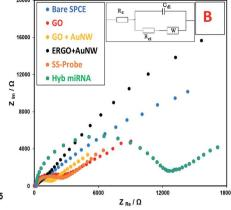
Fig. 2 Electrochemical analysis of the different stages of nanobiosensor preparation using (A) CV, and (B) EIS analysis in [Fe(CN)<sub>6</sub>]<sup>3-/4-</sup> solution.
