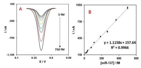
Fig. 4 (A) DPV analysis of the intercalated Dox on the hybridized target and SS-probe on the nanobiosensor for linear range concentrations of miR-137 from 5.0 to 750.0 fM (in a solution of PBS, pH 7.0). (B) Linear plot of Dox reduction peak current versus concentration of the target miR-137 (from 5.0 to 750.0 fM) (based on four replicates).
