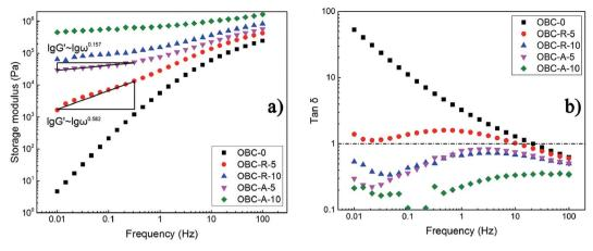
Fig. 4 Logarithmic plots of (a) the storage modulus and (b) the loss tangent as a function of frequency.
