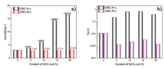
Fig. 3 (a) Dielectric permittivity and (b) dielectric loss for OBC/R974 and OBC/A200 nanocomposites at 1 Hz.
