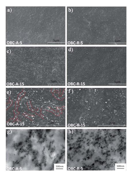
Fig. 1 Typical SEM micrographs of nanocomposites (a) OBC-A-5, (b) OBC-R-5, (c and e) OBC-A-15, (d and f) OBC-R-15, and typical TEM images of nanocomposites (g) OBC-A-5, (h) OBC-R-5.
