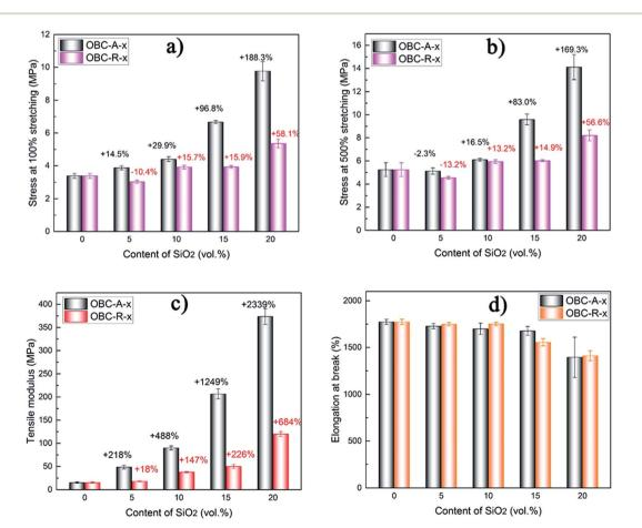
Fig. 5 (a) Stress at 100% stretching, (b) stress at 500% stretching, (c) elongation at break and (d) tensile modulus of OBC/R974 and OBC/A200 nanocomposites as a function of  $SiO_2$ . Percentages in (a), (b) and (c) are the percentages of reinforcement in stress at 100% stretching, stress at 500% stretching and tensile modulus, respectively when compared with pure OBC.
