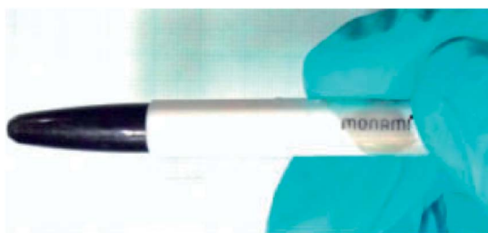
Fig. 22 Fully rollable graphene-based NG. 103
