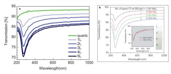
Fig. 49 (a) UV-vis optical transmittance for bare quartz and for different layers of graphene films on quartz. This figure has been adapted/ reproduced from ref. 167 with permission from Elsevier, (b) UV-vis spectra of transferred graphene films on quartz substrates. This figure has been adapted/reproduced from ref. 100 with permission from Nature Publishing Group.
