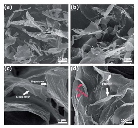
Fig. 35 (a) Low-magnification, (b and c) moderate-magnification, (d) high-magnification FESEM images of few-layer graphene. This figure has been adapted/reproduced from ref. 143 with permission from Elsevier.
