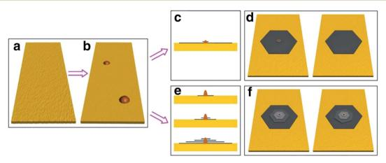
Fig. 63 The proposed mechanism for graphene domain growth. (a) Smooth Cu foil was obtained by cleaning in a pretreatment step. (b) Formation of large oxide nanoparticles on the pretreated Cu foil. (c and d) In high hydrogen concentration conditions, large-single-crystal monolayer graphene was formed. (e and f) In low hydrogen concentration conditions, multilayer graphene was obtained. This figure has been adapted/reproduced from ref. 199 with permission from Springer.
