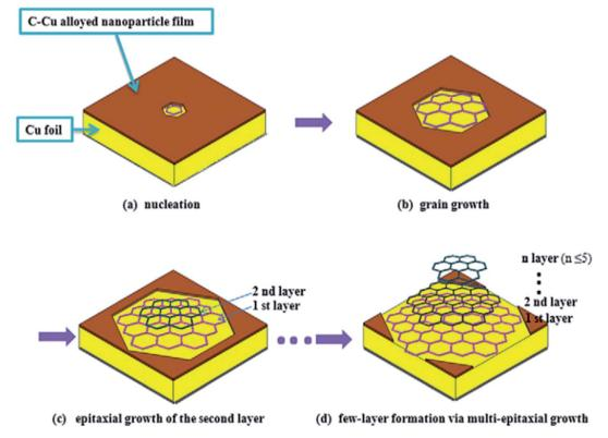
Fig. 68 Schematic of the growth of graphene domains on copper foil under APCVD conditions: (a) nucleated graphene grain, (b) the size of the graphene grain increases, (c) the second layer grows on the first layer epitaxially and (d) few-layer graphene produced by a multi-epitaxial growth. This figure has been adapted/reproduced from ref. 207 with permission from Elsevier.
