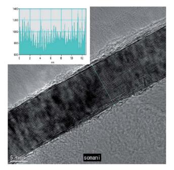
Fig. 1 High magnification TEM image of a planar few-layer graphene film. The inset shows the intensity pattern along the line marked. This figure has been adapted/reproduced from ref. 22 with permission from Elsevier.
