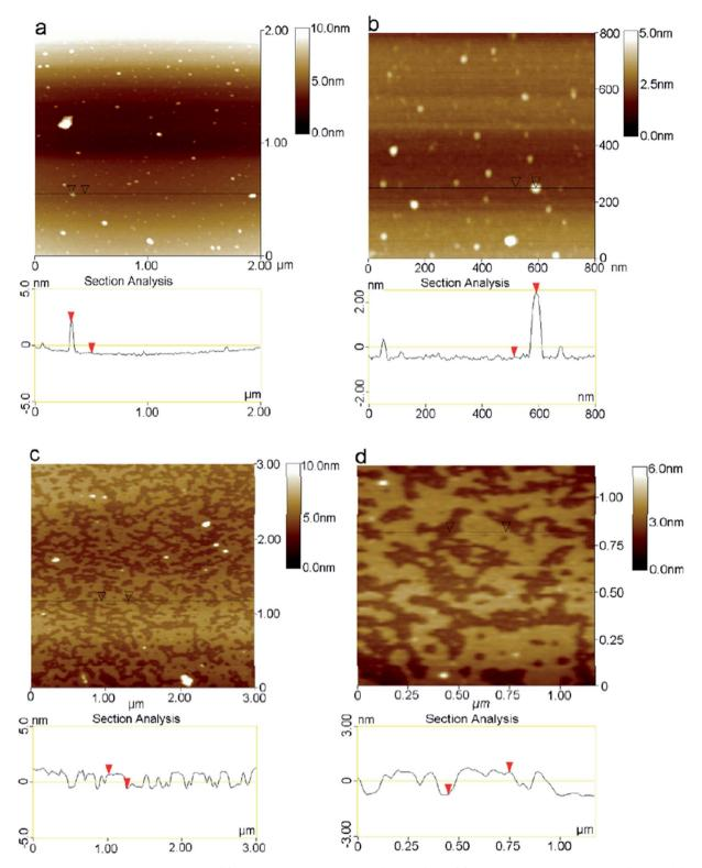
Fig. 53 Typical tapping mode AFM images of (a) few-layer graphene sheets 2  $\mu$ m  $\times$  2  $\mu$ m, (b) few-layer graphene sheets 0.8  $\mu$ m  $\times$  0.8  $\mu$ m, (c) monolayer graphene sheets 3  $\mu$ m  $\times$  3  $\mu$ m, and (d) monolayer graphene sheets 1.25  $\mu$ m deposited on the mica substrate from dispersion, corresponding height cross-sectional profile. This figure has been adapted/reproduced from ref. 90 with permission from Elsevier.
