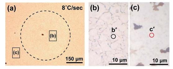
Fig. 56 (a) Low-magnification optical microscope image of as-synthesized graphene on Ni/SiO $_2$ /Si substrate using 2 sccm CH $_4$ , 30 s growth duration and a fast cooling process. (b)  $\theta$  (c) High-magnification images of the regions corresponding to the region in (a). Dashed circle in (a) presents a boundary where graphene is synthesized. This figure has been adapted/reproduced from ref. 179 with permission from Springer.
