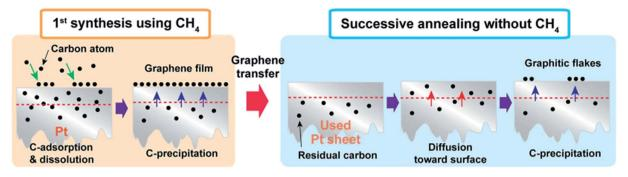
Fig. 59 Schematic of the formation of graphene and graphitic flakes by a carbon precipitation mechanism in Pt. This figure has been adapted/reproduced from ref. 179 with permission from Springer.
