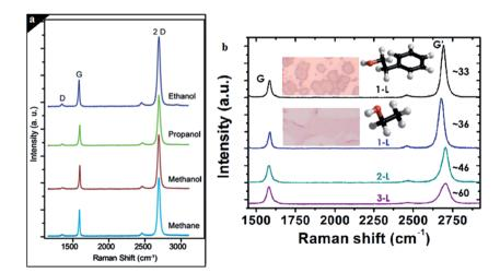
Fig. 4 (a) Comparison of the Raman spectra for graphene film synthesized by methanol, ethanol and 1-propanol. This figure has been adapted/ reproduced from ref. 66 with permission from Elsevier. (b) Raman spectra of single (black and blue lines for 2-phenylethanol and ethanol, respectively), bi (green line) and tri (purple line) layer graphene. This figure has been adapted/reproduced from ref. 61 with permission from Elsevier.
