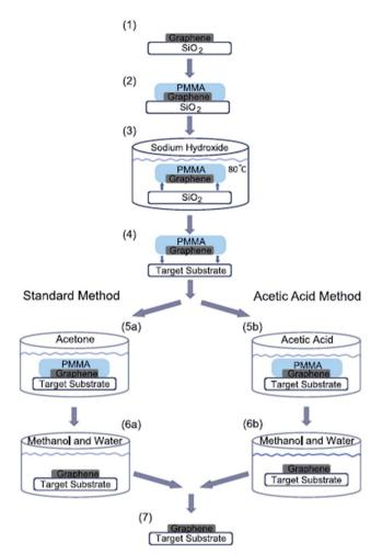
Fig. 13 Schematic of graphene transfer. PMMA was deposited on a graphene layer and cured at 115 °C for 2 min. The graphene-PMMA stack was then detached from the substrate in a sodium hydroxide bath and subsequently deposited on a target substrate. Finally, the PMMA was dissolved using acetone or acetic acid and then rinsed in a mixture of methanol and water. This figure has been adapted/ reproduced from ref. 104 with permission from Elsevier
