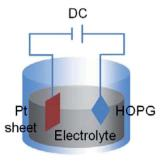
Fig. 8 Schematic of electrochemical exfoliation. This figure has been adapted/reproduced from ref. 75 with permission from The Materials Research Society of Japan.
