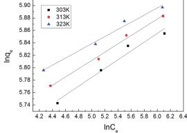
Fig. 11 Freundlich isotherm for MB removal using Cu-AC.
