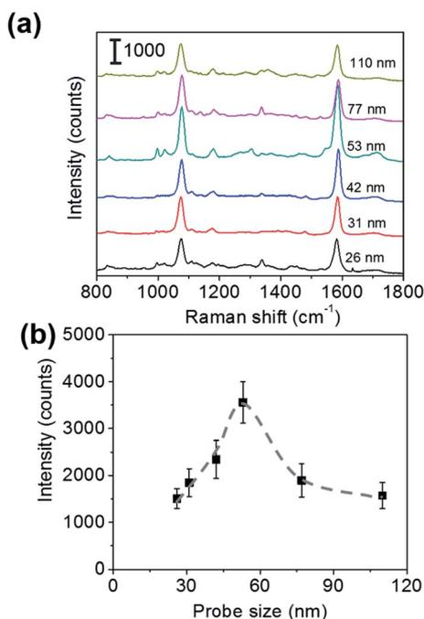
Fig. 2 (a) SERS spectra of the sandwich immunoassay for H-IgG performed at a constant H-IgG concentration of 1  $\text{ng mL}^{-1}$  using SERS probes of different sizes. (b) Probe size dependence of the SERS intensity of the 1587  $\text{cm}^{-1}$  band. The broken curve is a guide for the eye.
