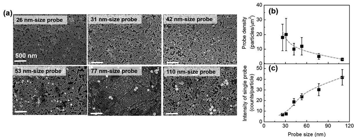
Fig. 4 (a) Representative SEM images of sandwich immunoassay substrates performed at a H-IgG concentration of  $1 \text{ ng mL}^{-1}$  using SERS probes of different sizes. Probe size dependence of (b) probe density and (c) SERS intensity of a single probe. The broken curves are guides for the eye.
