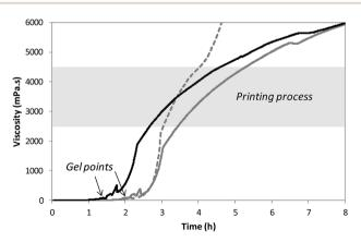
**Fig. 2** Viscosity of the hybrid solutions recorded as a function of time. Dashed grey line: hybrid PEG solution at 37 °C; solid grey line: hybrid PEG solution at 37 °C until gel point and then at 25 °C; black line: hybrid PEG–GRGDSP solution at 37 °C until gel point and then at 25 °C. Gels points were determined by rheology and reported on the viscosity curves.
