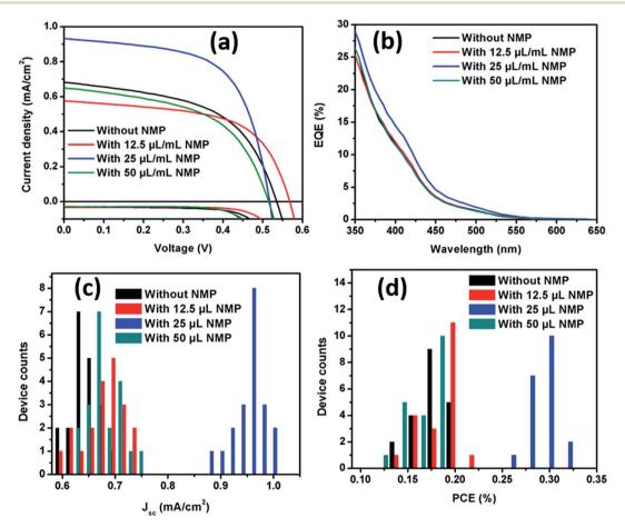
Fig. 3 (a) Average J-V curves, (b) IPCE spectra, (c)  $J_{sc}$  and (d) PCE histogram plot of devices containing MBI perovskite without and with different concentration of NMP.
