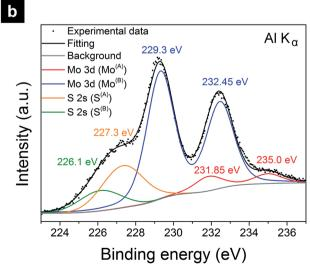
Fig. 2 Chemical analysis of the  $MoS_x/GCNT/CP$  electrode with XPS in (a) S 2p, and (b) Mo 3d-S 2s regions.
