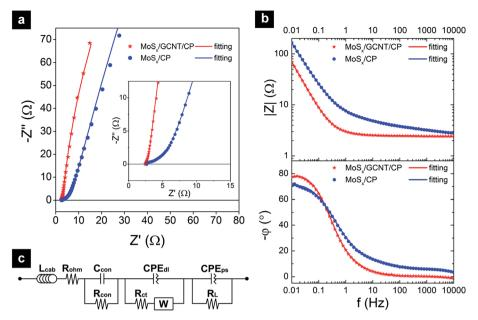
Fig. 6 EIS spectra and equivalent circuit fittings of the  $MoS_x/GCNT/CP$  and  $MoS_x/carbon$  paper electrodes presented in (a) Nyquist plot with (inset) the closed up view at high frequency region, and (b) Bode plots. (c) Equivalent circuit used for all fittings in (a, b).
