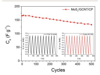
Fig. 7 Degradation test of the  $MoS_x/GCNT/CP$  electrode performed with 500 charge/discharge cycles at 5 A  $g^{-1}$ , showing the degradation of electrode specific capacitance during the test, with (insets) plots of the first and last 10 charge/discharge cycles (time axes t are referenced to the beginning of each 10-cycle set).
