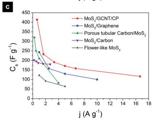
Fig. 5 Supercapacitive performance of electrodes assessed by galvanostatic charge/discharge curves. (a) Charge/discharge curves of the MoS<sub>x</sub>/GCNT/CP electrode obtained at different charge/discharge rates from 0.67 to 16.7 A  $g^{-1}$ . (b) The dependence of electrode specific capacitance on charge/discharge rate. (c) A comparison of the discharge capacitance of MoSx/GCNT/CP against crystalline MoS2based electrode materials reported in the literature.
