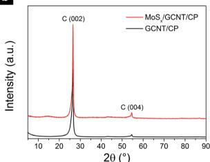
Fig. 3 Crystallinity analyses of the  $MoS_x/GCNT/CP$  electrode with (a) Raman spectroscopy, and (b) XRD.
