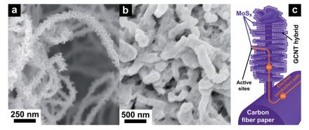
Fig. 1 Morphological characterization with FE-SEM of (a) the GCNT/CP support, and (b) the MoS<sub>x</sub>/GCNT/CP electrode. (c) Schematic illustration of the MoS<sub>x</sub>/GCNT/CP electrode structure.
