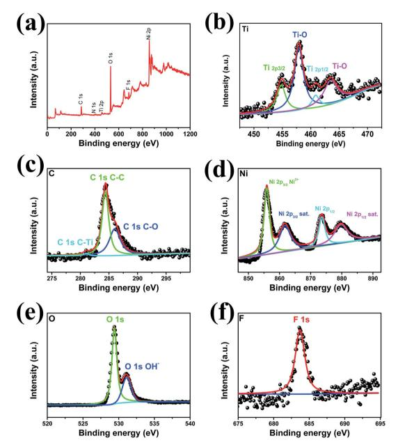
Fig. 3 (a) High-resolution XPS survey spectra. (b) Ti 2p, (c) C 1s, (d) Ni 2p, (e) O 1s, and (f) F 1s spectra of Ni-dMXNC
