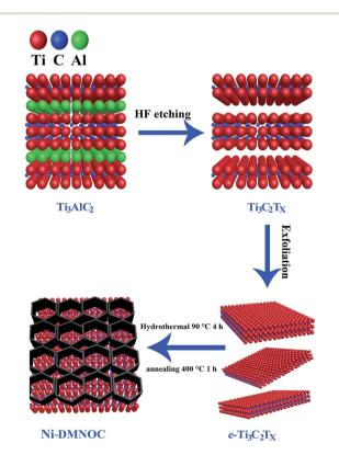
$\begin{tabular}{lll} Scheme 1 & Schematic of the preparation of the Ni-dMXNC by facile hydrothermal method. \\ \end{tabular}$
