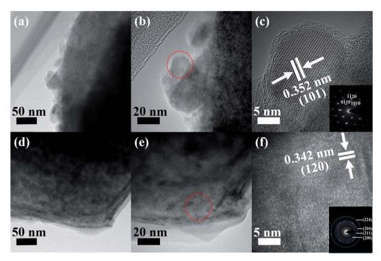
Fig. 4 (a) and (b) Low-magnification TEM image, (c) HRTEM image (red circle area in (b)), and corresponding SAED pattern (inset) of the  $Ti_3C_2T_x$  MXene; (d) and (e) low-magnification TEM image, (f) HRTEM image (red circle area in (e)), and corresponding SAED pattern (inset) of the Ni-dMXNC.
