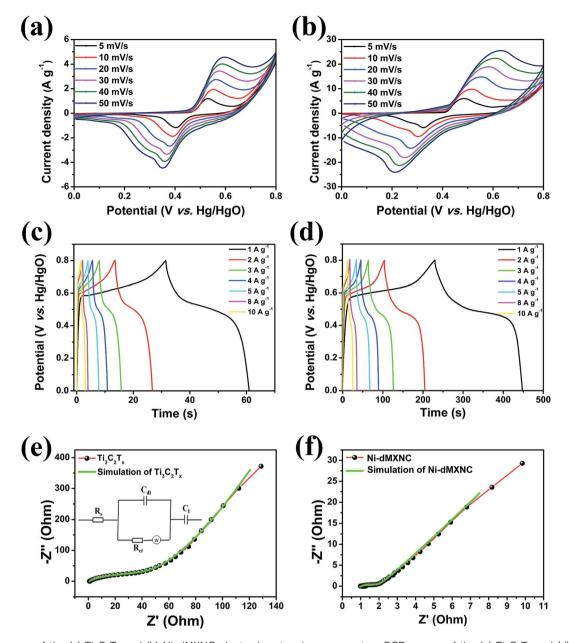
Fig. 5 CV curves of the (a)  $Ti_3C_2T_x$  and (b) Ni-dMXNC electrodes at various scan rates; GCD curves of the (c)  $Ti_3C_2T_x$  and (d) Ni-dMXNC electrodes at various scan rates and current densities. EIS of the (e)  $Ti_3C_2T_x$  and (f) Ni-dMXNC electrodes.
