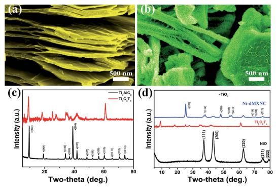
Fig. 1 SEM images of the (a) as-obtained  $Ti_3C_2T_x$  MXene after DMSO treatment, and (b) the as-obtained Ni-dMXNC. (c) XRD patterns of pre-HF-treated  $Ti_3AlC_2$  MAX phase and post-HF treated  $Ti_3C_2T_x$  MXene. (d) XRD patterns of NiO nanosheets,  $Ti_3C_2T_x$  MXene, and Ni-dMXNC.
