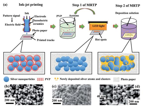
Fig. 3 (a) Schematic representation of MRTP. SEM images show the morphologies of the silver tracks at different steps. (b) Before sintering, (c) treated by the Step 1 of MRTP and (d) treated by Step 2 of MRTP. The inset in (d) shows the high resolution image of small nanoparticles newly deposited on to the silver track.
