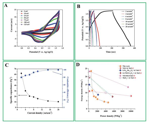
Fig. 6 (A) CV curves of ASC fabricated using Ni/Ni(OH)<sub>2</sub>//AC at various scan rates; (B) galvanostatic charge/discharge (GCD) curves of ASC at various current densities. (C) Specific capacitance and coulombic efficiency as function of current density for ASC; (D) Ragone plot comparison with previous reports.
