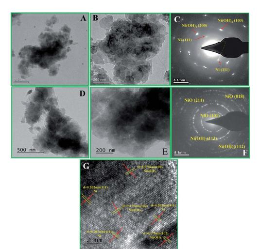
Fig. 3 (A and B) Transmission electron microscopic (TEM) images of  $Ni/Ni(OH)_2$  NS at lower and higher magnification; (C) the corresponding SAED pattern; (D and E) TEM images of  $NiO/Ni(OH)_2$  NS at lower and higher magnification; (F) the corresponding SAED pattern and (G) high resolution TEM image of  $Ni/Ni(OH)_2$  NS.
