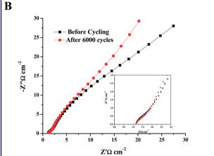
Fig. 7 (A) Cyclic performance of ASC at  $15 \text{ mA cm}^{-2}$  for 6000 cycles. Inset: CV curves at a scan rate of  $5 \text{ mV s}^{-1}$  before and after 6000 cycles. (B) Nyquist plots of the ASC cell before and after cycling; inset: high frequency region of Nyquist plot.
