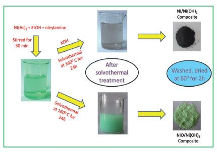
Scheme 1 Schematic representation of Ni/Ni(OH)<sub>2</sub> and NiO/Ni(OH)<sub>2</sub> NSs synthesis, and visible observations.
