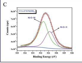
Fig. 2 (A) X-ray photoelectron spectra (XPS) of the survey of Ni/Ni(OH)<sub>2</sub> NS; (B) XPS of the Ni 2p state of Ni present in Ni/Ni(OH)<sub>2</sub> NSs. (C) XPS of O 1s state of O present in Ni/Ni(OH)<sub>2</sub> NSs.
