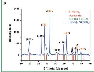
Fig. 1 (A and B) X-ray diffraction (XRD) patterns of the synthesized Ni/Ni(OH) $_2$  and NiO/Ni(OH) $_2$  NSs.
