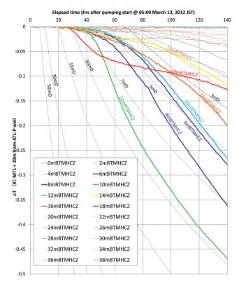
Fig. 14 Estimated temperature drop for various permeabilities (k = 3– 50 mD) at the location r = 20 m and measured the temperatures of selected depths in the reservoir of the AT1-MT1 borehole.
