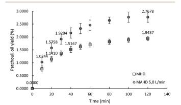
Fig. 4 Comparison between the yields of patchouli oil obtained by microwave hydrodistillation and microwave air-hydrodistillation (air flow rate 5.0 L min<sup>-1</sup>). The microwave power was 600 W and the ratio of patchouli leaves to distilled water was 0.10 g mL<sup>-1</sup>.
