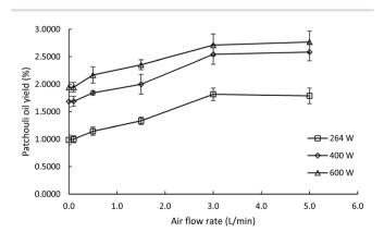
Fig. 3 The effect of the air flow rate on the yield of patchouli oil extracted at different microwave power levels. The ratio of patchouli leaves to distilled water was  $0.10~{\rm g~mL^{-1}}$ .
