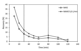
Fig. 6 Recovery of patchouli oil obtained by microwave hydrodistillation (MHD) and microwave air-hydrodistillation (MAHD; air flow rate 5.0 L min<sup>-1</sup>). The microwave power was 600 W and the ratio of patchouli leaves to distilled water was 0.10 g mL<sup>-1</sup>.
