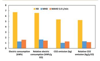
Fig. 9 The electric consumption and environmental impact ( $CO_2$  emissions) for the extraction of patchouli oil by the conventional method (hydrodistillation; HD), the microwave hydrodistillation method (MHD) and the microwave air-hydrodistillation method (MAHD; air flow rate 5.0 L min<sup>-1</sup>). The microwave power was 600 W and the ratio of patchouli leaves to distilled water was 0.10 g mL<sup>-1</sup>.
