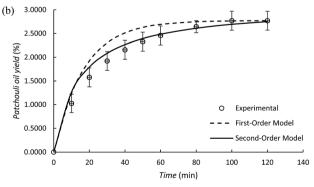
Fig. 7 A comparison of the first-order and second-order kinetic models with the experimental results for the extraction of patchouli oil by (a) microwave hydrodistillation and (b) microwave air-hydrodistillation (air flow rate  $5.0 L min^{-1}$ ). The microwave power was 600 Wand the ratio of patchouli leaves to distilled water was  $0.10 \text{ g mL}^{-1}$ .
