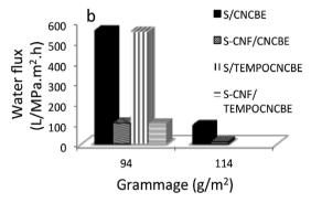
Fig. 6 Water flux of fabricated support layers with and without  ${\sf CNF}_{\sf SL}$  (a) with different grammage. Layered fabricated membranes indicate the decrease in water flux (b) but *in situ* TEMPO oxidation has no significant effect on water flux (b).
