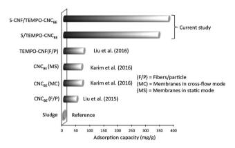
Fig. 7 A comparative study of adsorption capacity of Cu(n) with different operation parameters with two nanocellulose (CNF and  $CNC_{BE}$ ). Sludge was taken as reference in the current study. The highest adsorption capacity was recorded for *in situ* functionalized membranes as discussed in current study.
