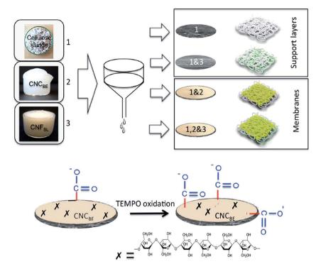
Fig. 1 Schematic representation of the processing of support layers and membranes. Support layer of sludge and  $CNF_{SL}$  were fabricated using 1<sup>st</sup> filtration. Functional layers on support layers were fabricated using 2<sup>nd</sup> filtration. Numbers 1, 2 and 3 indicate the sludge, functional nanocellulose  $(CNC_{BE})$ , and  $CNF_{SL}$  respectively. Schematic representation of *in situ* functionalization of top layer (below) is shown. Symbol **X** represent cellulose chain.
