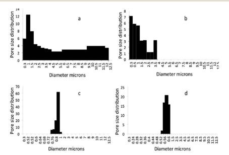
Fig. 5 Pore-size distributions of support layers having sludge (a) and mixture of sludge and CNF<sub>SL</sub> (b). Layered membranes fabricated using second filtration on sludge support layer (c) and hybrid of sludge and CNF<sub>SL</sub> (d) showed lower and narrow pore size distribution.
