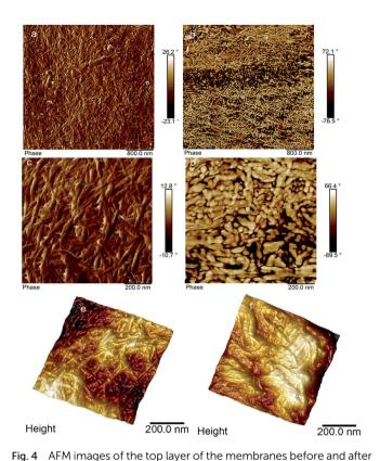
in situ modifications. (a and c) Shows the phase images at different magnifications and (e) shows the 3D height images of  $CNC_{BE}$  layer. (b, d and f) Shows the corresponding phase images at different magnifications and the 3D height images of  $CNC_{BE}$  layer after in situ TEMPO modification.
