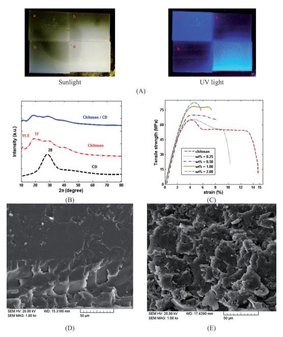
Fig. 4 (A) Photographic images of a: chitosan/CDs nanocomposites and b: chitosan film under sunlight and UV light (366 nm). (B) XRD patterns of CDs, chitosan and chitosan/CDs nanocomposites. (C) Stress-strain curves for chitosan and chitosan/CDs nanocomposites films. (D) Typical SEM micrograph of chitosan and (E) 1.0 wt% chitosan/CDs nanocomposites films.
