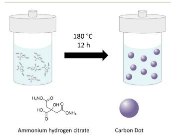
Scheme 1 Schematic illustration for synthesis of carbon dots.
