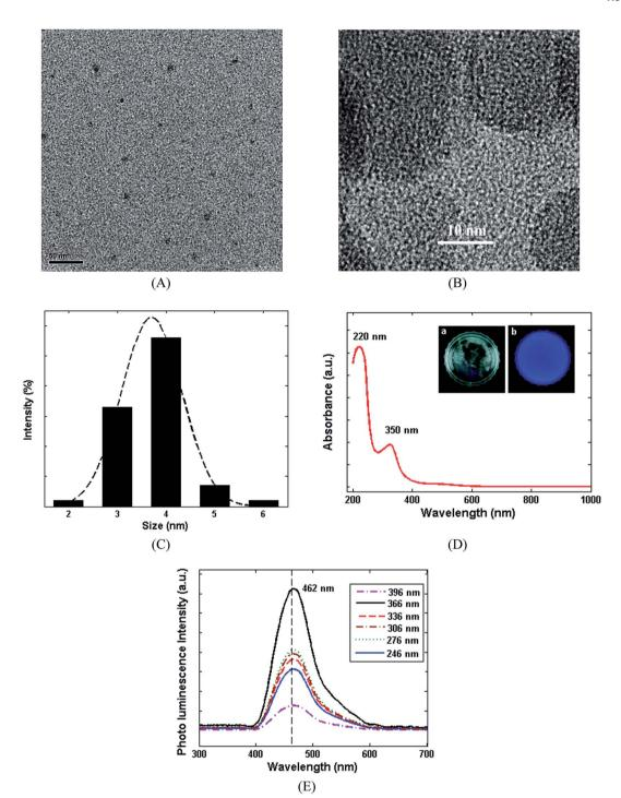
Fig. 1 (A) TEM and (B) HRTEM images of CDs. (C) Particle size distribution of CDs, (D) UV-Visible absorption spectrum of CDs. The insets: photographic images of the CDs (1 mg ml $^{-1}$ ) under a: sunlight and b: UV light (366 nm). (E) PL response of the CDs by varying the excitation wavelength from 246 to 396 nm.
