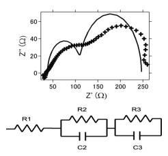
Fig. 8 (a) Nyquist plot of the intact aluminum—air battery with the aircathode materials being activated carbon (AC) before electrochemical reaction. (b) Equivalent circuit of present aluminium air battery.
