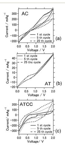
Fig. 3 Cyclic voltammograms of the aluminum-air battery with the air-cathode materials (a) AC (b) AT and (c) ATCC.
