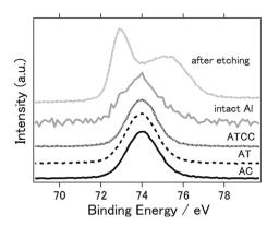
Fig. 6 X-ray photoelectron spectra of Al 2p of aluminium anode before (intact aluminium), after etching, and after the electrochemical reaction (AC, AT, ATCC).
