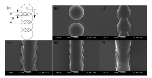
Fig. 3 Wax line structures jetted with these parameters: degree of overlap 0 to 80%, voltage 40 V, frequency 11 Hz, and nozzle diameter 75  $\mu$ m, (a) schematic of the droplet overlap, (b) k = 0, (c) k = 10%, (d) k = 30%, (e) k = 50%, (f) k = 80%.
