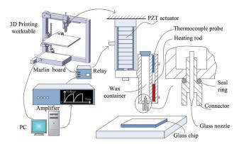
Fig. 1 Schematic of the 3D wax printing system.
