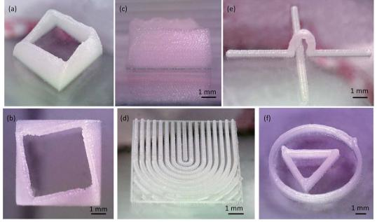
Fig. 6 3D printed wax structures photographed through a handheld microscope, (a) isometric view of the spirally growing square shell, (b) plane view of the shell, (c) elevation view of the shell, (d) 3D letter U shape, (e) bridge model for real 3D fluid channels, (f) 3D printed triangular and circular structures.
