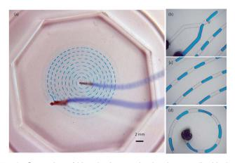
Fig. 8 Generation of blue dyed water droplets in corn oil with the spiral micro channel at a feed speed of 2  $\mu$ L min<sup>-1</sup>, (a) global view, (b) pressure induced breaking of water in the inlet area, (c) spiral flow of the droplets, (d) outlet area.
