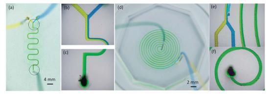
Fig. 7 3D printed micromixers mixing blue and yellow dyes (a) mixing in the winding microchannel at a feeding speed of  $10~\mu$ L min $^{-1}$ . Areas in the black circles are magnified in (b) and (c), (b) magnified inlet junction, (c) magnified fluid channel near the outlet, (d) mixing in the spiral microchannel at a feed speed of  $100~\mu$ L min $^{-1}$ , (e) magnified spiral microchannel inlet junction, (f) magnified fluid channel near the spiral microchannel outlet.
