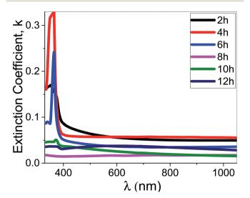
Fig. 10 The extinction coefficient for the synthesized films at different deposition time as a function of the wavelength.
