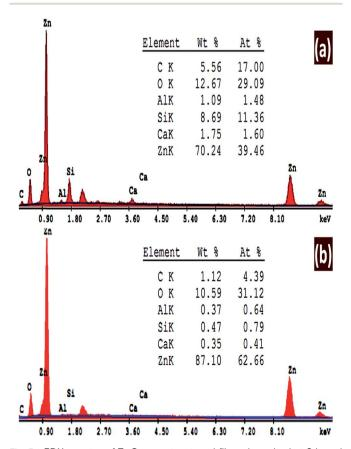
Fig. 5 EDX spectra of ZnO nanostructured films deposited at 8 h and pH (a) 6.5 and (b) pH 7.
