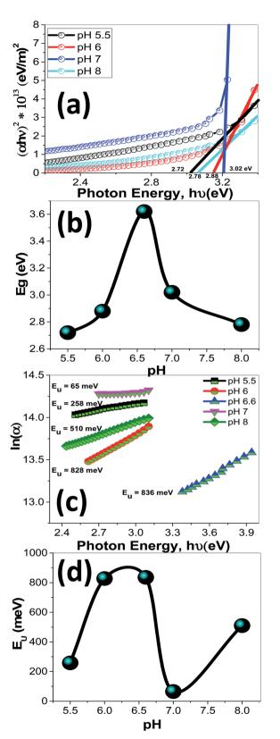
Fig. 14 The plots of (a)  $(\alpha h \nu)^2 \ \theta \ h \nu$  to determine  $E_{\rm g}$  values, (b)  $E_{\rm g}$  as a function of pH, (c)  $\ln(\alpha) \ \theta \ h \nu$  to determine Urbach energy ( $E_{\rm U}$ ), and (d)  $E_{\rm U}$  as a function of pH for nanostructured ZnO films.
