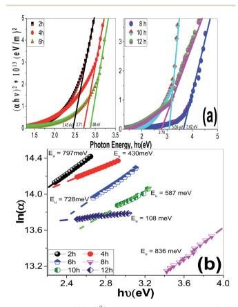
Fig. 11 The plots of (a)  $(\alpha h \nu)^2 + h \nu$  to determine  $E_{\rm g}$  values and (b)  $\ln(\alpha) + h \nu$  to determine to determine the Urbach energy of ZnO films of different morphologies.
