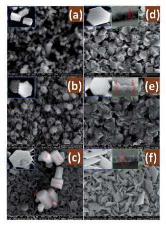
Fig. 6 SEM images of nanostructured ZnO thin films deposited at different times (a) 2, (b) 4, (c) 6, (d) 8, (e) 10 and (f) 12 h. The insets showed magnified and cross-sectional SEM images.
