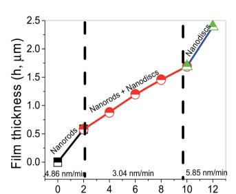
Fig. 7 Variation of film thickness with deposition time.
