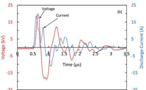
Fig. 2 Typical voltage and current waveforms for (a) Cyl-d-DBD and (b) PtP-d-DBD reactors.
