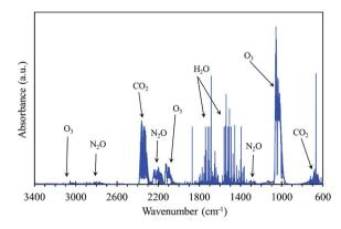
Fig. 3 Typical gas phase FTIR spectrum acquired during DW treatment using Cyl-DBD reactor at room temperature and atmospheric pressure:  $1 \text{ L min}^{-1}$  air, 20.5 kV and 400 Hz.
