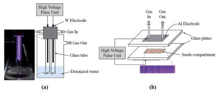
Fig. 1 Schematic of the plasma reactors for (a) water activation and (b) seeds treatment.
