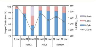
Fig. 7 Micelle shape distribution (spherical, ellipsoidal and rod-like micelles) in growth solutions at different Hofmeister salt concentrations and the L-LSPR<sub>max</sub> of the rods grown in those solutions.
