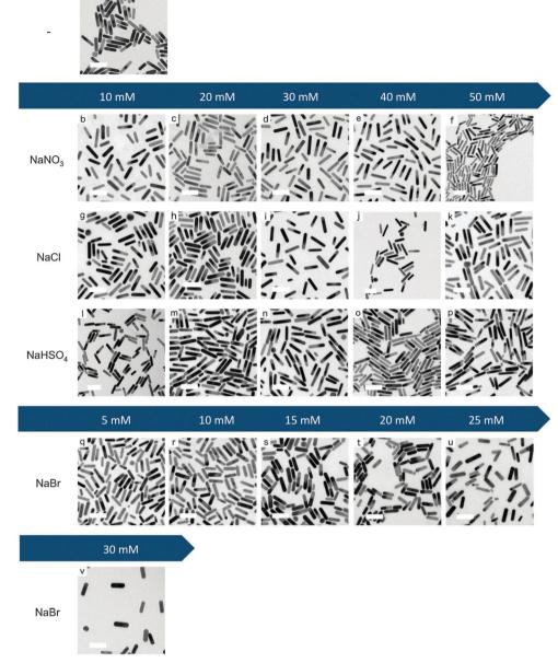
Fig. 2 TEM images of Au NRs synthesized using our seed-mediated method with different amounts of Hofmeister salts: (a) without Hofmeister salts, (b-f) with NaNO<sub>3</sub>, (q-k) with NaCl and (l-p) with NaHSO<sub>4</sub> in the order of increasing added concentration (10-50 mM), and (q-v) with NaBr in the order of increasing added concentration (5-30 mM). All scale bars are 50 nm.
