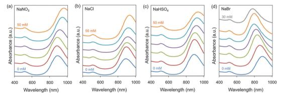
Fig. 1 Normalized extinction spectra of Au NRs grown in the presence of additional amounts of Hofmeister salts. For (a) – (c) the salt concentrations are 0 mM (blue), 10 mM (red), 20 mM (green), 30 mM (purple), 40 mM (turquoise) and 50 mM (orange) from bottom to top. For (d), the salt concentrations are 0 mM (blue), 5 mM (red), 10 mM (green), 15 mM (purple), 20 mM (turquoise), 25 mM (orange) and 30 mM (grey) from bottom to top. All the spectra have been offset for easier comprehension
