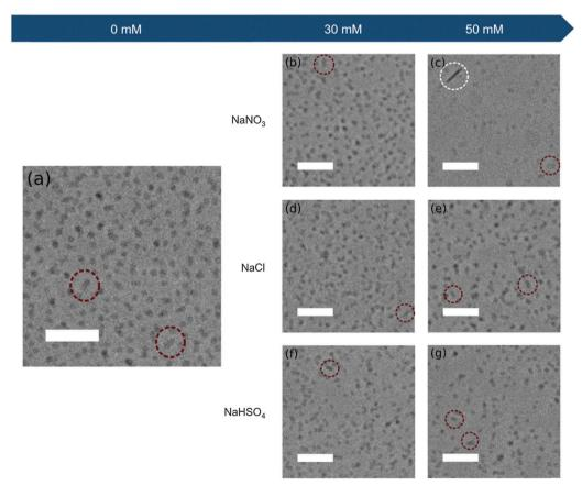
Fig. 6 Cryo-TEM images of CTAB micelles in the growth solutions with different amounts of Hofmeister salts: (a) without Hofmeister salts, (b and c) with NaNO<sub>3</sub>, (d and e) with NaCl and (f and g) with NaHSO<sub>4</sub> in the order of increasing added concentration (30 and 50 mM). Some ellipsoidal and rod-like micelles have been highlighted in red and white dashed circles, respectively. All scale bars are 50 nm.
