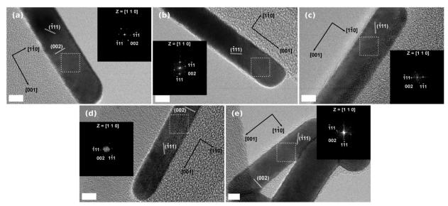
Fig. 3 HR-TEM images of Au NRs synthesized (a) without Hofmeister salts, (b) with NaNO<sub>3</sub> (50 mM), (c) with NaCl (50 mM), (d) with NaHSO<sub>4</sub> (50 mM) and (e) with NaBr (30 mM). The insets in the images are the fast Fourier transform patterns of the selected regions. All scale bars are 5 nm.
