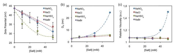
Fig. 5 (a) Zeta potential, (b) hydrodynamic diameter and (c) the relative viscosity of growth solutions in the presence of added Hofmeister salts.
