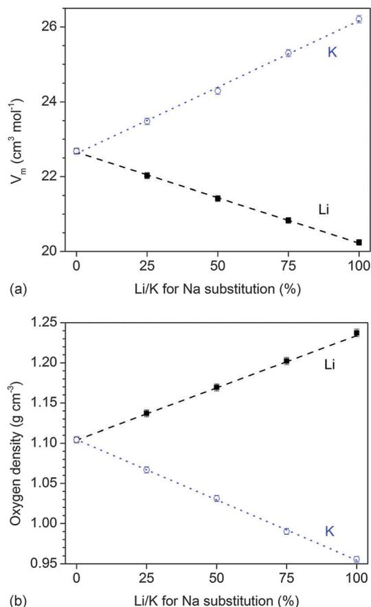
Fig. 8 (a) Molar volume,  $V_m$ , and (b) oxygen density, a parameter describing the compactness of the silicate network, vs. Li/K for Na substitution in the glass. Lines are linear regression:  $R^2(V_m) = 0.999$  (Li),  $0.998$  (K);  $R^2(\text{oxygen density}) = 0.999$  (both Li and K).
