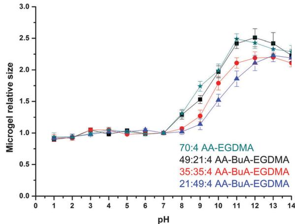
Fig. 7 Swelling ratios of the AA–BuA–EGDMA microgels and the AA–EGDMA microgel at different pH values. Microgels formed with AA:BuA:EGDMA molar ratios of 70:0:4, 21:49:4, 35:35:4, 49:21:4 are represented as green stars, blue triangles, red circles and black squares, respectively.
