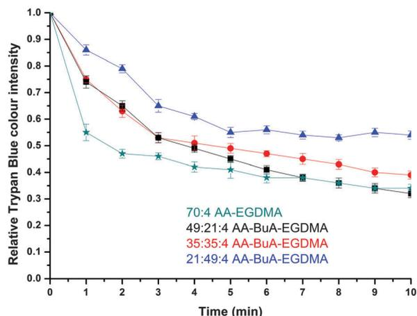
Fig. 12 Hydrophilic dye release in basic pH solution ( $\sim$ pH 11). The plots show the relative Trypan Blue colour intensity versus time for all AA–BuA–EGDMA microgels with different AA–BuA ratios and the AA homopolymer, AA–EGDMA. Green stars, black squares, red circles and blue triangles represent the microgels with 70:4, 49:21:4, 35:35:4 and 21:49:4 AA:BuA:EGDMA molar ratios, respectively.
