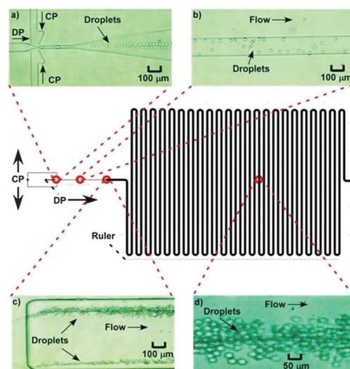
Fig. 6 Photographs of droplets (a) being generated at the flow focusing junction, (b) in the  $10 \mu\text{m}$  deep channel, (c) entering the  $60 \mu\text{m}$  deep serpentine channel, and (d) inside the serpentine channel where they would undergo UV polymerisation.
