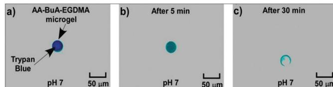
Fig. 10 Hydrophilic Trypan Blue encapsulation in, and release from, a AA<sub>49</sub>-co-BuA<sub>21</sub>-co-EGDMA<sub>4</sub> microgel (a) immediately following encapsulation and suspension in pH 7 solution, (b) 5 min later, and (c) 30 min after suspension in pH 7 solution.
