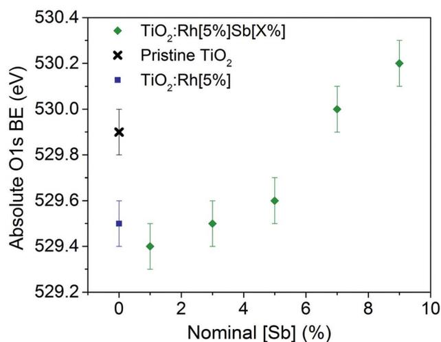
Fig. 4 Oxide O 1s absolute binding energy vs. nominal amount of Sb dopant. As  $\text{O}^{2-}$  is assumed chemically unchanged in the doped systems by comparison with pristine  $\text{TiO}_2$ , the observed variation in oxide O 1s binding energy can be attributed to movement of the Fermi level, which provides the 0 eV binding energy reference in XPS.
