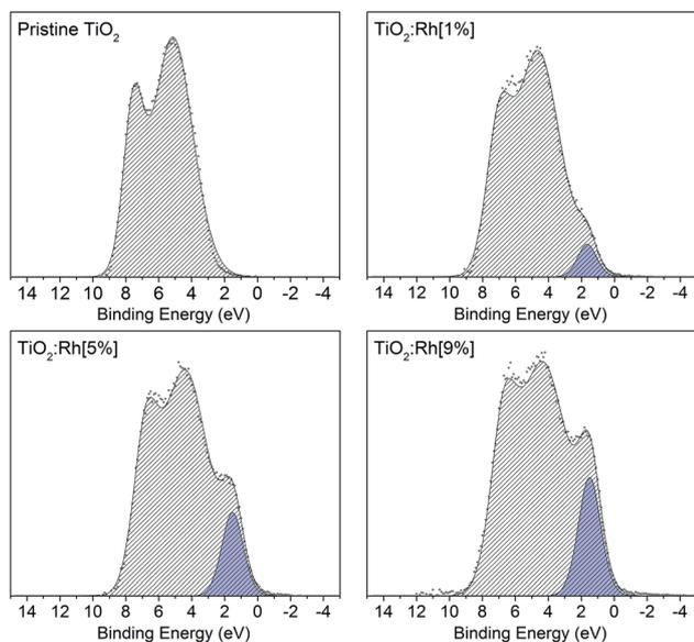
Fig. 3 Valence band spectra of pristine  $\text{TiO}_2$  and 1, 5 and 9% Rh doped  $\text{TiO}_2$ . As the nominal amount of Rh increases, the prominence of an in-gap feature due to Rh 4d  $t_{2g}$  electrons also increases.
