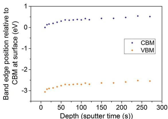
Fig. 7 VBM and CBM variation with depth in a Sb/Rh codoped TiO<sub>2</sub> (110) crystal. The CBM at the surface is placed at 0 eV and the band gap is assumed to be 3.06 eV as in bulk rutile TiO<sub>2</sub>. The Sb/Rh dopant ratio was measured by XPS depth profiling. This was correlated with the Fermi level shifts as described in the text.
