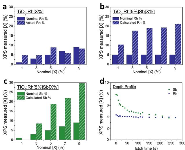
Fig. 2 (a–d) Dopant percentage amount as determined from XPS; (a) Rh in  $\text{TiO}_2:\text{Rh}$ , (b) Rh in  $\text{TiO}_2:\text{RhSb}$  and (c) Sb in  $\text{TiO}_2:\text{RhSb}$ , (d) depth profile showing atomic% of Rh and Sb as determined by XPS spectra taken after intervals of etching with an  $\text{Ar}^+$  ion gun.
