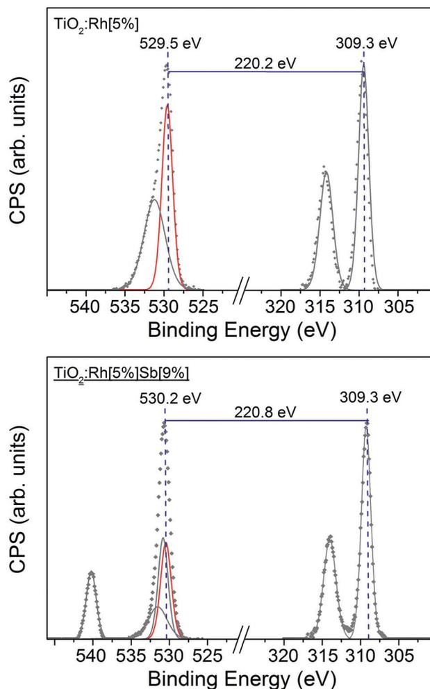
**Fig. 5** Binding energy separation between O 1s and Rh 3d peaks in TiO<sub>2</sub>:Rh[5%] (top) and TiO<sub>2</sub>:Rh[5%]Sb[9%] (bottom). The energy difference between the corelines increases with Sb doping. Assuming a static oxide O 1s peak with no chemical shift, the increasing energy difference upon Sb doping is attributed to a decrease in the binding energy of the Rh 3d coreline, corresponding to a less positive oxidation state for Rh.
