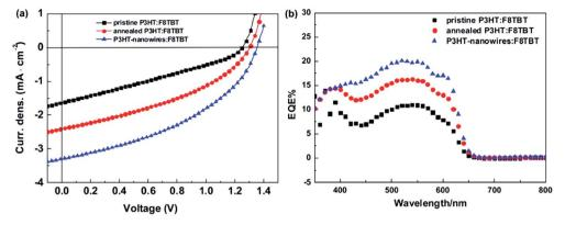
Fig. 21 (a) J-V characteristics and (b) EQE spectra of the as-cast P3HT/F8TBT (black squares), annealed P3HT/F8TBT (red circles), and P3HT-nanowire/F8TBT (blue triangles) blend solar cells under simulated AM1.5G solar light illumination with an intensity of 100 mW cm<sup>-2</sup>. Both the annealed P3HT/F8TBT and P3HT-nanowire/F8TBT blends were annealed at 140 °C for 15 min before electrode deposition. Reproduced with permission from (ref. 53). Copyright 2014, American Chemical Society.
