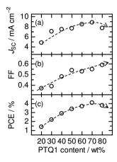
Fig. 18 Photovoltaic parameters ( $J_{SC}$ , FF, PCE) of PTQ1/N2200 blend solar cells with various D : A ratios. The broken lines are guides for the eye. Reproduced with permission from (ref. 51). Copyright 2013, Wiley-VCH Verlag GmbH & Co. KGaA, Weinheim.
