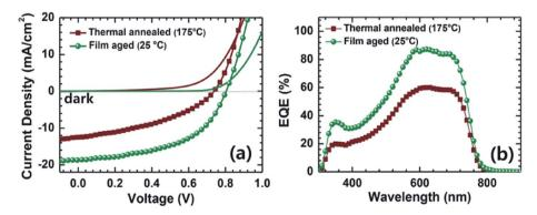
Fig. 13 (a) J-V curves and (b) EQE spectra of PTB7-Th/PNDIS-HD (1:1 w/w) blend solar cells with thermally annealed (175 °C, 10 min) or filmaged (25 °C, 72 h) active layers. Adapted with permission from (ref. 76). Copyright 2015, Wiley-VCH Verlag GmbH & Co. KGaA, Weinheim.
