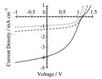
Fig. 9 J-V characteristics of P3HT/PF12TBT solar cells under AM 1.5G 100 mW cm $^{-2}$  illumination. The devices were fabricated *via* spincoating from DCB (dotted line), CB (dashed line), and CF (solid line) solutions of P3HT and PF12TBT (1: 1 weight ratio) and annealed at 140 °C for 10 min. Adapted with permission from (ref. 41). Copyright 2011, American Chemical Society.
