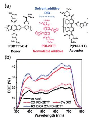
Fig. 12 (a) Chemical structures of the PBDTTT-C-T donor, P(PDI-DTT) acceptor, PDI-2DTT, and DIO. (b) EQE spectra of PBDTTT-C-T/ P(PDI-DTT) blend solar cells without or with additives under AM 1.5G solar simulator illumination at 100 mW cm<sup>-2</sup>. Reproduced with permission from (ref. 56). Copyright 2013, The Royal Society of Chemistry.
