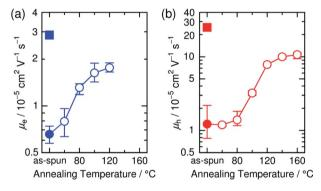
Fig. 15 (a) Electron and (b) hole mobilities of P3HT/PF12TBT blend films (circles) with respect to annealing temperature. The squares in (a) and (b) indicate the electron and hole mobilities, respectively, of the as-spun PF12TBT neat and as-spun P3HT neat films. Reproduced with permission from (ref. 91). Copyright 2015, Wiley-VCH Verlag GmbH  $\vartheta$  Co. KGaA, Weinheim.
