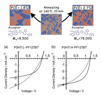
Fig. 16 J-V characteristics of (a) P3HT/L-PF12TBT and (b) P3HT/H-PF12TBT blend solar cells under AM 1.5G illumination from a calibrated solar simulator with an intensity of 100 mW cm<sup>-2</sup>. The device was fabricated by spin-coating a CF solution of P3HT and PF12TBT (1:1 weight ratio) and annealed at 100 °C (broken lines) and 140 °C (solid lines) for 10 min. Reproduced with permission from (ref. 46). Copyright 2012, American Chemical Society.
