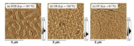
Fig. 10 AFM phase images of P3HT/PF12TBT blend films spin-coated from (a) DCB (b) CB, and (c) CF solutions of P3HT and PF12TBT (1:1 weight ratio), on glass substrates and annealed at 140 °C for 10 min.
