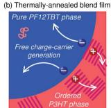
Fig. 26 Illustration of the nanoscale morphology of polymer phase separation; (a) the as-spun and (b) thermally annealed P3HT/PF12TBT blend films.
