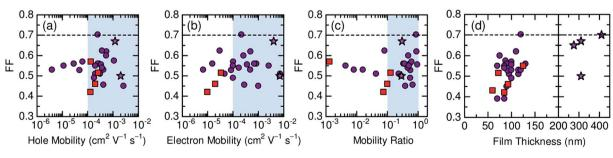
Fig. 29 Plots of (a) hole and (b) electron mobilities measured in the blend film *versus* FF measured in solar cells composed of PDI-based (squares) and NDI-based (circles and stars) polymer acceptors. (c) Mobility ratio, defined as the ratio of the slower carrier mobility to the faster carrier mobility, *versus* corresponding FF. (d) Plots of device film thickness *versus* corresponding FF.
