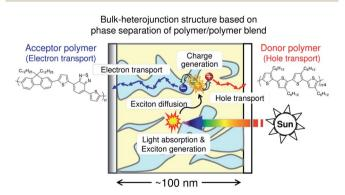
Fig. 1 Photovoltaic conversion processes in polymer/polymer blend solar cells: (1) exciton generation *via* photon absorption; (2) exciton diffusion at a donor/acceptor interface; (3) charge transfer at the interface and charge dissociation into free charge carriers; and (4) charge transport to each electrode.
