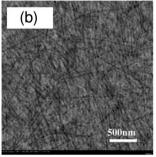
Fig. 20 Transmission electron microscopy images of the (a) P3HT/ F8TBT blend film prepared from DCB and (b) P3HT-nanowire/F8TBT blend film prepared from a mixed solution of DCB and n-hexane. The scale bar corresponds to a length of 500 nm. All the blend films have a thickness of  $\sim$ 80 nm. Reproduced with permission from (ref. 53). Copyright 2014, American Chemical Society.
