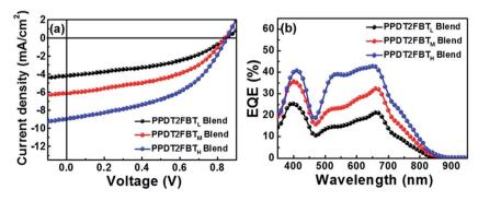
Fig. 17 (a) J-V characteristics and (b) EQE spectra of PPDT2FBT/P(NDI2OD-T2) blend solar cells. Adapted with permission from (ref. 71). Copyright 2015, American Chemical Society.
