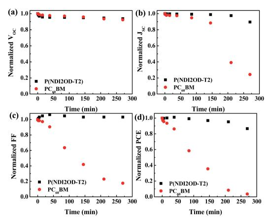
Fig. 4 Variation with time of (a)  $V_{OC}$ , (b)  $J_{SC}$ , (c) FF and (d) PCE of the HPSCs using P(NDI2OD-T2) and PC<sub>60</sub>BM as EELs.
