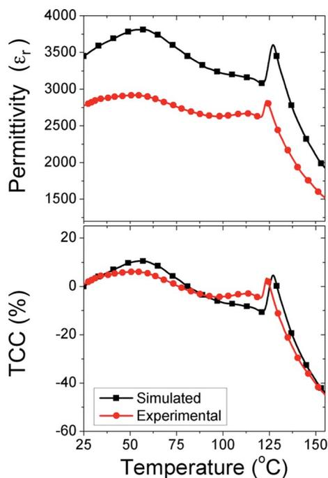
Fig. 6 Overlaid FEM simulation models and experimental data of temperature profiles for (a)  $\epsilon_r$  and (b) TCC. Excellent agreement is obtained showing the prediction of combining a BT core with 2.5% doped NNBT with  $V_f = 0.66$  provides potentially useful TCC behaviour.
