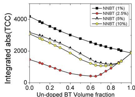
Fig. 5 The integrated absolute TCC response versus  $V_f$  of undoped BT for NNBT-BT ceramics based on Fig. 1. This provides a new method to identify the best combination of doped materials with undoped BT to minimise TCC in MLCCs.
