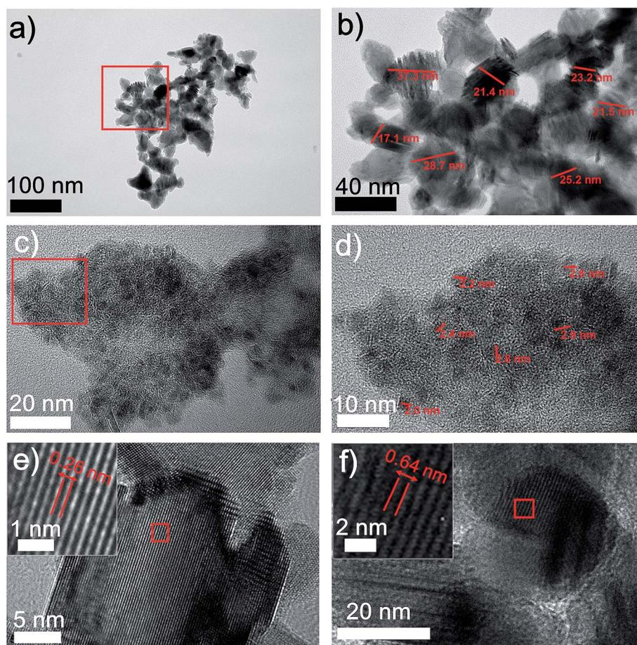
Fig. 2 (a) and (b) TEM images of MoS<sub>2</sub> NPs in the laser-induced MoS<sub>2</sub>/carbon hybrids; (c) and (d) TEM images of MoS<sub>2</sub> QDs in the laser-induced MoS<sub>2</sub>/carbon hybrids; (e) and (f) HRTEM images of MoS<sub>2</sub> NPs in the laser-induced MoS<sub>2</sub>/carbon hybrids. Inset images show their lattice spacings of 0.26 and 0.64 nm, indicating the (200) and (100) planes of MoS<sub>2</sub> NPs.
