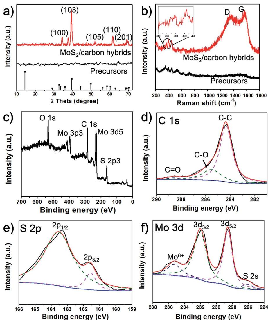
Fig. 3 (a) XRD spectra of the laser-induced MoS<sub>2</sub>/carbon hybrids and their precursors; (b) Raman spectra of the laser-induced MoS<sub>2</sub>/carbon hybrids and their precursors; (c) XPS survey of the laser-induced MoS<sub>2</sub>/carbon hybrids. (d), (e), and (f) high-resolution XPS spectra of C 1s, S 2p and Mo 3d, respectively.
