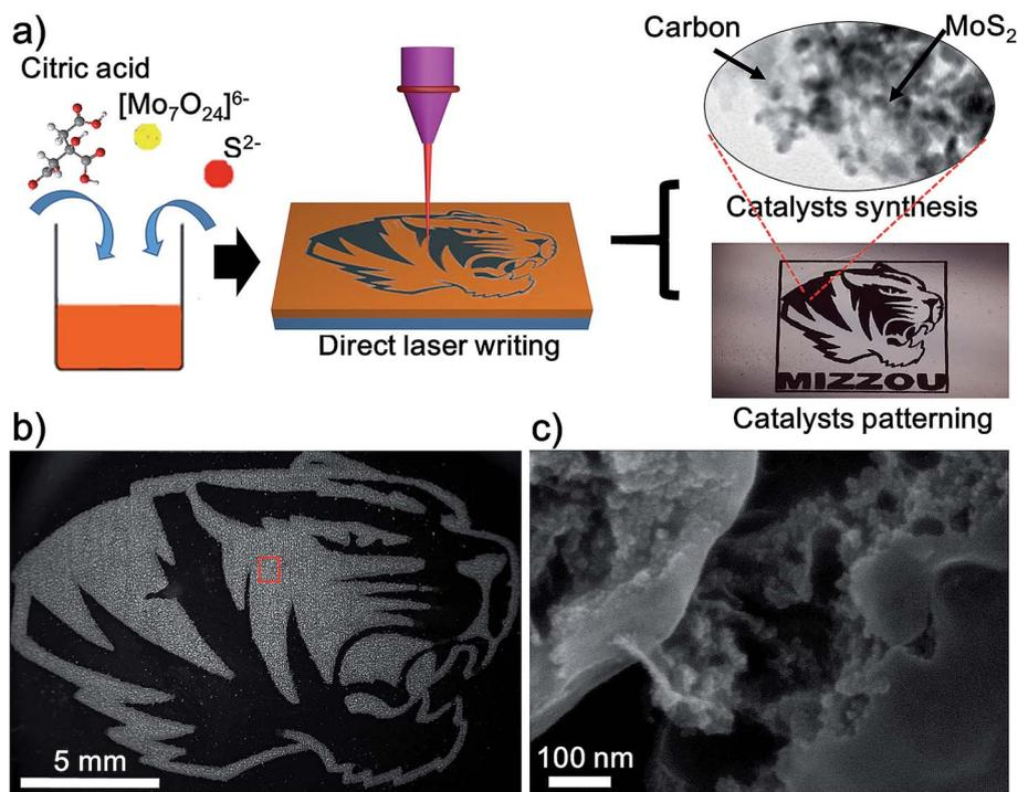
Fig. 1 (a) Scheme of the DLW method in fabricating arbitrary patterns composed of MoS<sub>2</sub>/carbon hybrids. (b) SEM image of a patterned Mizzou tiger logo composed of MoS<sub>2</sub>/carbon hybrids. (c) Magnified SEM image of the selected area indicated in (b).
