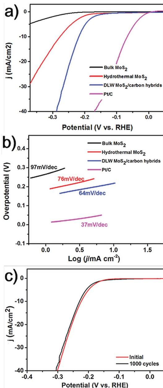
Fig. 4 (a) Polarization curves of Pt/C, bulk MoS<sub>2</sub>, hydrothermal MoS<sub>2</sub>, and laser induced MoS<sub>2</sub>/carbon hybrids. (b) Tafel plots of Pt/C, bulk MoS<sub>2</sub>, hydrothermal MoS<sub>2</sub>, and laser induced MoS<sub>2</sub>/carbon hybrids. (c) Polarization curves of laser induced MoS<sub>2</sub>/carbon hybrids before and after 1000 cycles of CV sweeping.
