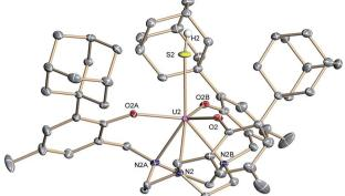
Fig. 1 Molecular structure of the uranium(IV) hydrosulfido complex  $[((^{Ad,Me}ArO)_3tacn)U-SH]$  (2) with the chalcogen-bound H atom located in the difference Fourier map. All other hydrogen atoms and the solvent molecules are omitted for clarity (50% probability ellipsoids).
