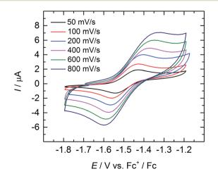
Fig. 5 Quasi-reversible oxidation wave of 3 at different scan rates. Measurement conducted in THF with  $\sim$ 0.1 M [N(n-Bu) $_4$ ][BPh $_4$ ] electrolyte, using Fc $^+$ /Fc couple as internal standard.
