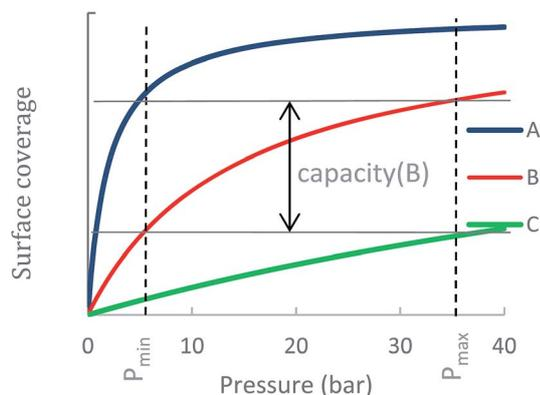
Fig. 1 Usable capacity of three different ANG materials A, B and C, where  $\Delta H_{\text{ads}}(\text{A}) > \Delta H_{\text{ads}}(\text{B}) > \Delta H_{\text{ads}}(\text{C})$ . The usable capacity is proportional to the difference between surface coverage at maximal and minimal pressures. The usable capacity of B is larger than A and C since A is over-adsorbing and C is under-adsorbing.
