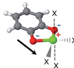
**Fig. 4** The catechol-Mg metalated linker. The electrostatic dipole moment (arrow) is formed by the two negatively charged O atoms and the positive metal. 'X' marks potential CH<sub>4</sub> adsorption sites. The positive and negative formal charges are marked by red and blue colors, respectively.
