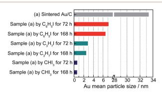
Fig. 4 Au average particle size of sintered Au/C before and after redispersion by different iodohydrocarbons for 72 h and 168 h, as indicated by TEM images in Fig. S9.†
