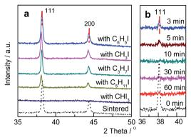
Fig. 1 (a) XRD patterns of sintered Au/C catalyst and after treatment with various iodohydrocarbons 40  $^{\circ}$ C for 3 h; (b) XRD patterns of sintered Au/C catalyst before and after treatment with CHI<sub>3</sub> at 40  $^{\circ}$ C as a function of time.
