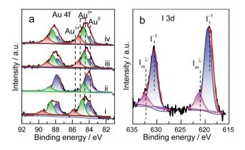
Fig. 3 (a) Au 4f XPS spectra of Au/C catalysts after treatment under different conditions: (i) as-prepared; (ii) sintered; (iii) sintered Au/C treated with CHI3 at 40 °C for 30 min; and (iv) redispersed Au/C (sample (iii)) activated by HCl gas at 150 °C for 30 min. (b) I 3d XPS spectra of the redispersed Au/C catalyst (sample (iii)).
