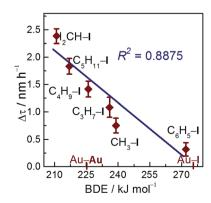
Fig. 5 Correlation plots of the dependence of C–I BDEs of iodohydrocarbons on Au NP redispersion rate at 40  $^{\circ}$ C, derived from variations in radius of Au NPs before and after treatment with iodohydrocarbons.
