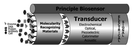
Fig. 10 Elements and components of a typical biosensor (figure by author)
