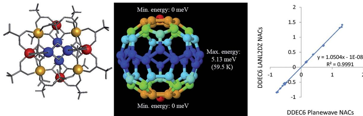
Fig. 9 Left: Atomic structure of Mn<sub>12</sub>-acetate single molecule magnet. Mn type 1 (blue), Mn type 2 (red), Mn type 3 (yellow). In the minimum energy conformations, the Mn ASM vectors are perpendicular to the plane of the page. Middle: Computed spin-orbit coupling potential energy surface. Right: Comparison of DDEC6 NACs computed with LANL2DZ and planewave basis sets.
