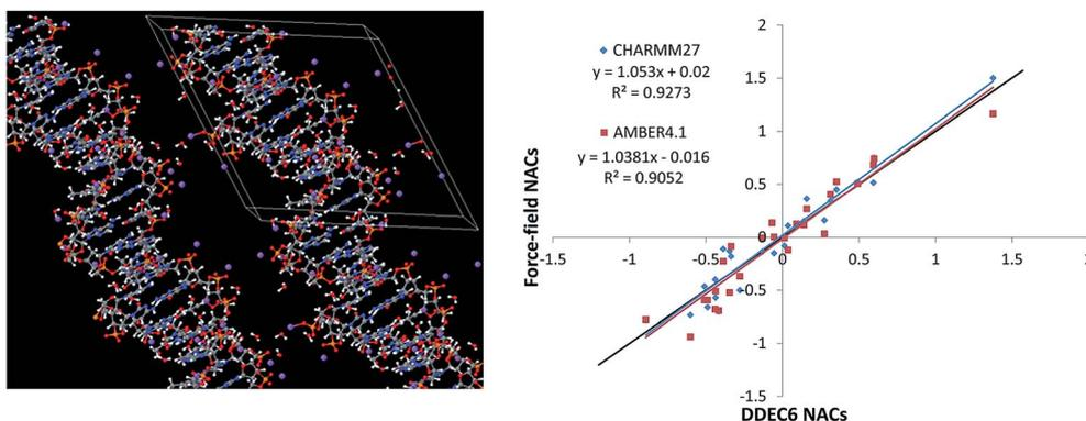
**Fig. 5** Left: B-DNA decamer (CCATTAATGG)<sub>2</sub>, the lines mark the unit cell boundaries. Right: Correlation between DDEC6, CHARMM, and AMBER force-field NACs for all atoms excluding the bound water molecules and added Na<sup>+</sup> atoms. The black line has a slope of 1 and intercept of 0. CHARMM27 NACs from Foloppe and Mackerell.<sup>82</sup> AMBER4.1 NACs from Cornell *et al.*<sup>85</sup>
