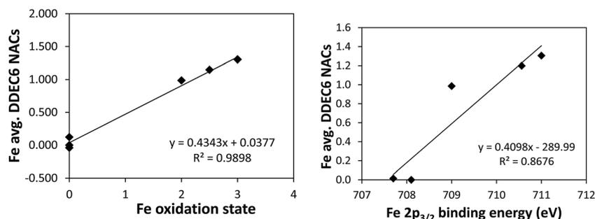
Fig. 4 Left: Correlation between Fe oxidation state and average Fe DDEC6 NAC for Fe, Fe<sub>2</sub>SiO<sub>4</sub>, Fe<sub>2</sub>O<sub>3</sub>, Fe<sub>3</sub>O<sub>4</sub>, and Fe<sub>3</sub>Si solids. Right: Correlation between 2p<sub>3/2</sub> core electron binding energy (as measured using XPS) and average Fe DDEC6 NAC for these materials.
