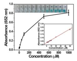
Fig. 5 Dependence of the absorbance at 652 nm on the concentration of  $\rm H_2O_2$  from 1  $\mu M$  to 1 mM. The upper and lower insets show the corresponding photographs of different solutions and linear calibration plot, respectively.
