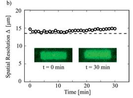
Fig. 4 Intensity profile a) of the activated pattern (inset) averaged along the direction y. The width  $\Delta$  of the transition region (grey area) is a measure of the spatial resolution of the DROPLAY technique. The parameter  $\Delta$  is approximately equal to the mean droplet diameter (dashed line in panel b) and slightly increases over the time due to the slow leakage of caged fluorescein across adjacent droplets. Scale bar is 50 μm.
