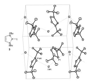
Fig. 2 Molecular structure and representation of the unit cell of crystalline 2-iodo-1,3-di-t-butyl-1,3,2-diazaphospholene (3). Interactions between DAP fragments and iodine atoms parallel to the crystallographic b-axis are represented as dashed lines. Selected distances (Å) I(1)-P(1) 3.426(1), I(1)-P(1)#1 3.558(1). Reproduced with permission from ref. 21. Copyright 2009 Wiley-VCH Verlag GmbH & Co. KGaA.
