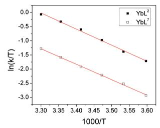
Fig. 6 Eyring plots for  $YbL^2$  and  $YbL^7$  in  $D_2O$  for the exchange of fluoride-bound and hydrated complexes.
