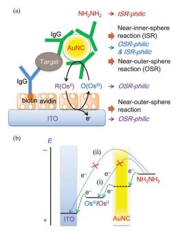
Fig. 1 (a) Schematic of an immunosensor using outer-sphere to innersphere electrochemical-nanocatalytic (EN<sub>c</sub>) redox cycling. (b) Schematic of three-step electron transfer related to EN<sub>c</sub> redox cycling (green lines) and unwanted electron transfer (sky-blue lines). The applied potential, the formal potentials of  $Os^{III}(bpy)_2Cl_2^+/Os^{II}(bpy)_2Cl_2$  and hydrazine, and the potential of the Au nanocatalyst (AuNC) (horizontal lines) are positioned in order of potential.
