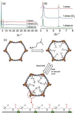
Fig. 1 (a) Synchrotron PXRD profiles of 1-dmen, 1-dmen-CO<sub>2</sub>, and 1-dmen-re. (b) Enlargement of the low-angle region of the PXRD data. (c) Framework structure of 1 with open metal sites, grafting modes of dmen onto the open metal sites, and subsequent  $CO_2$  adsorption. The schematic diagram (bottom) indicates the arrangement of ammonium carbamates running along the c-axis.
