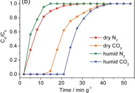
Fig. 5 (a)  $CO_2$  adsorption–desorption cycling curve for **1-dmen** in humid conditions. (b) Breakthrough curves for **1-dmen** under dry ( $N_2$ , red circle;  $CO_2$ , orange circle) and humid conditions ( $N_2$ , green triangle;  $CO_2$ , blue triangle).
