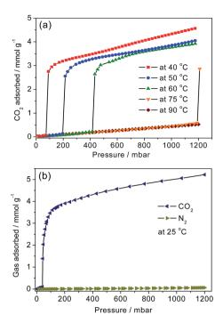
Fig. 2 (a) Adsorption isotherms of CO<sub>2</sub> for 1-dmen at the indicated temperatures. The solid lines are eye-guides. (b)  $CO_2$  and  $N_2$  isotherms at 25 °C.
