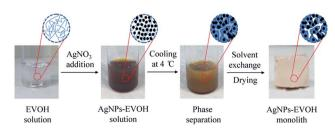
Fig. 1 A general procedure for fabrication of AgNPs-EVOH monolith.
