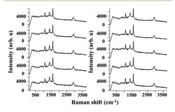
Fig. 4 Series of SERS spectra measured in the randomly selected 10 places on the AgNPs-EVOH monoliths.
