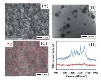
Fig. 3 SEM (A), TEM (B) and EDX (C) (red spots represent the existence of AgNPs) images of AgNPs–EVOH monolith. SERS spectrum (—) of R6G collected from the monolith and Raman spectrum (—) of the monolith (without R6G) (D).
