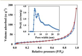
Fig. 2 Nitrogen adsorption/desorption isotherms of AgNPs-EVOH monolith. Adsorption points are marked by blue tetragons and desorption points by dark red tetragons.
